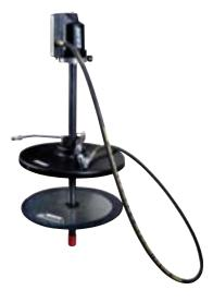
8. Turn on your air supply and press reset button. Hold the grease control valve near waste container (to collect test grease) and squeeze trigger. The air motor will function and test grease will appear followed by air (in the high pressure grease hose), then start greasing. Let go of the trigger: the pump should stop. Check for any grease leaks at hose connections. Tighten the connections as required.
