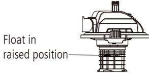
**IMPORTANT:** To reduce the risk of damage to the vac, do not run motor with float in raised position.
