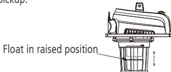
**IMPORTANT:** To reduce the risk of damage to the vac, do not run motor with float in raised position.
