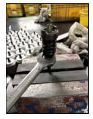
**5.** Adjust the torque/clutch of the hex nut with a 17mm hex wrench.
