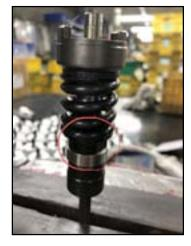
**4.** Locate the hex nut which is under the spring. (parts no.37).
