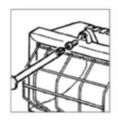
Unscrew retaining screw on top of lamp. This will release the protective grill, front surround and glass faceplate
