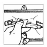
To insert halogen tube: unwrap bulb, taking care your fingers do not touch the bulb. Use wrapping to handle the bulb. Push one end of tube into either of the spring-loaded sockets. Locate other end on other socket, and release.
